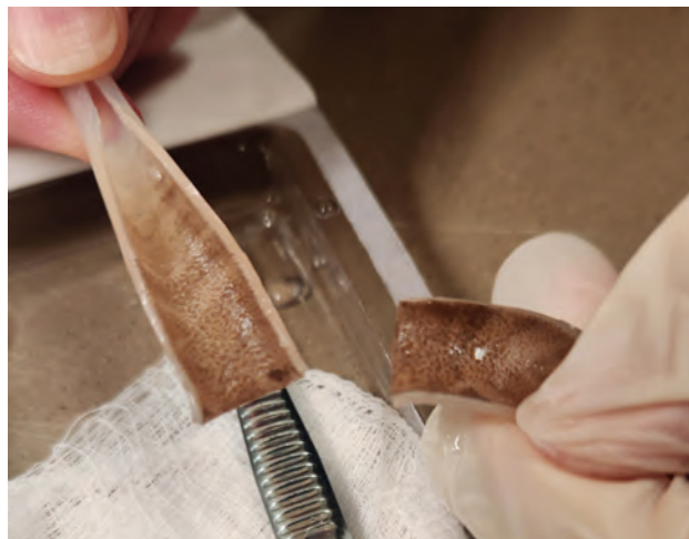
Picture 1: Bisected transfer set with brown discoloration
